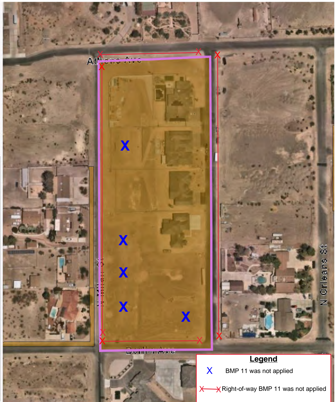
MAP 1 - Showing location that does not meet BMP 11 - Long-Term Stabilization Requirements.
